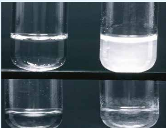
LAL test. Test tubes on the left are control samples of LAL; on the right, endotoxin has been added. The upper panel shows gel formation. The lower panel shows flocculent that forms early in the clotting reaction or in samples containing low concentrations of endotoxin.
